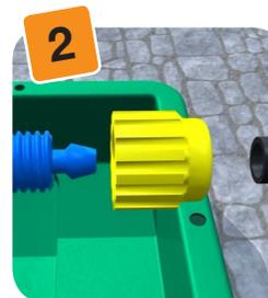
2.1 Remove the yellow collar from the AQUAvalve nozzle. Thread one end of the 6mm pipe through the yellow collar.
